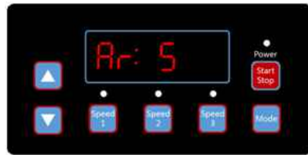
(Diagram 6.26, Auto Recovery count down, 5 seconds remaining) (图6.26, 自动复位倒数, 还剩5秒)
